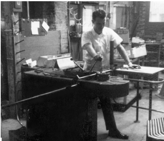
Dick founded Tube Specialties Company in 1963, bending tubing by hand to create fuel and brake hydraulic lines for trucks and tractors.
